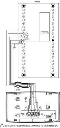
FOUR WIRES ARE REQUIRED FOR PROPER OPERATION. IF FEWER THAN FOUR ARE AVAILABLE, ADDITIONAL WIRES MUST BE RUN TO PC8900 LOCATION. IF MORE THAN FOUR ARE AVAILABLE, TAPE OFF UNUSED WIRES
